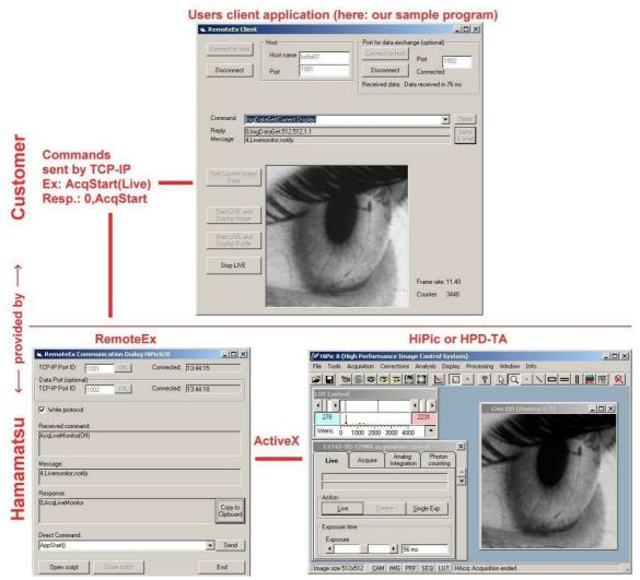
Schematic diagram of how the RemoteEx works.
